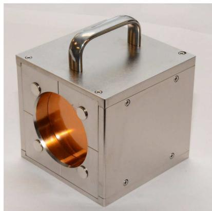
Prototype MLFC assembly with 128 layers of 0.0508 mm copper, suitable for proton beam energies up to 250 MeV. The assembly weighs 5.6 kg (12.2 lb) and measures 120 x 120 x 145 mm. The sheets are fully screened inside the housing and the signals are brought out on two VHDCI68 connectors. The useful area is 72 mm diameter, sufficient for the beam size of most PBS systems.
